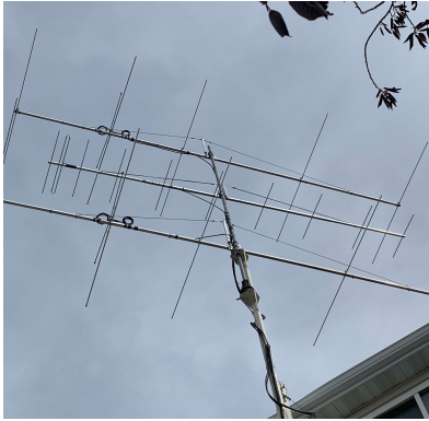
A single 10el OWL G/T (middle) at K7TNT - "Its doing well, Will let you know more after more testing. It is very well made"
