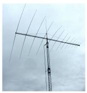
The 10-54MHz LDPA directional antenna at K4ANP. Sadly, Len caught one of the elements and bent it during installation but SWR 1:1.4 thorughout.
