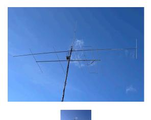
A highly efficient yet very HD 20m/14MHz rotating dipole
