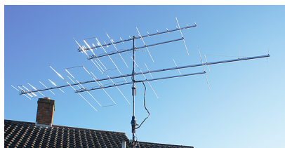
The 13el 144MHz LFA (second bottom) installed at G4VPD
