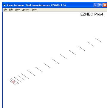
The 222MHz 14el LFA element layout
