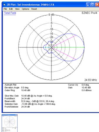
A High-Gain 24MHz LFA Yagi
