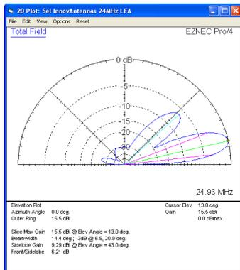
Single 5 element LFA up 12m above ground
