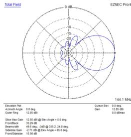
Above, Azimuth and elevation plots of a single 7el OWL Ultra on 144.1MHz. Note how tight the rear lobes are. Below elevation plot @ 10m above ground with ground reflections and ground gain.
