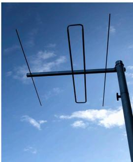
**A 3el Graves LFA Yagi ready for connection to a receiver.**
