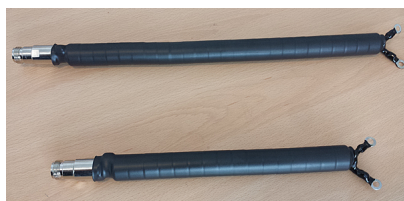
Examples of the InnovAntennas ferrite core baluns
