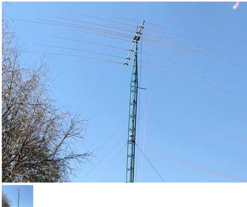
XR7 - 14 element 7 band HF, 6m & 4m Yagi(20/17/15/12/10/6/4) with 3.6m boom - The World's shortest 6 band HF & 6m & 4m Yagi 'full sized' Yagi - InnovAntennas
