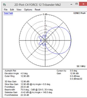
6m azimuth plot when placed 20m above ground. Note 13.39dBi including ground gain
