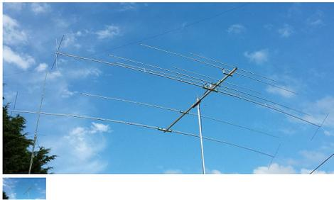
XR4 - 8 element 4 band HF & 6m Yagi (20/15/10/6) with 3.5m boom
