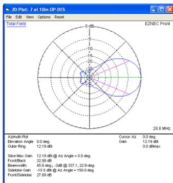
Azimuth plot at 28.6MHz
