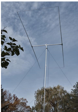
20m Moxon installed @ WA2TDE below
