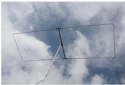
20m Moxon installed @ WA2TDE below
