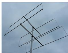
**A 3 element LFA-Q (Super-rigid Quad-style) Super-Light Quad Style Yagi for 144-146MHz**
