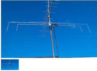
A three band low-loss rotating dipole for 15/10/6m Radiating efficiency like never seen before!
