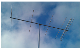
A 6 element OWL (Optimised Wideband Low Impedance) Super-Light Yagi for 69.9-70.5MHz
