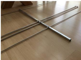
The super-light OWL's have elements connected and through the boom with a single securing bolt (3el rear mount OWL featured above)
