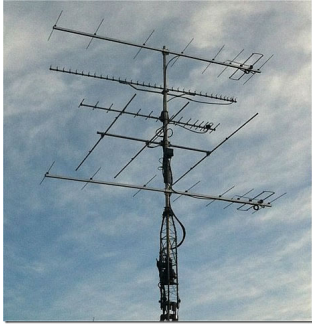
2 x 8el 144MHz LFA installed at G1MHU
