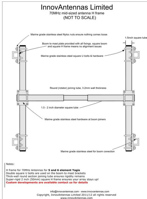
An H frame for 4 x 6el 70MHz LFA Yagis
