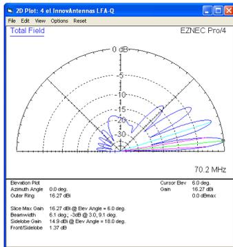
**Single 4 element LFA up 10m above ground**
