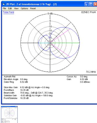
A low-noise 70MHz LFA2 Yagi
