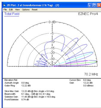
**Single 2 element LFA up 10m above ground**
