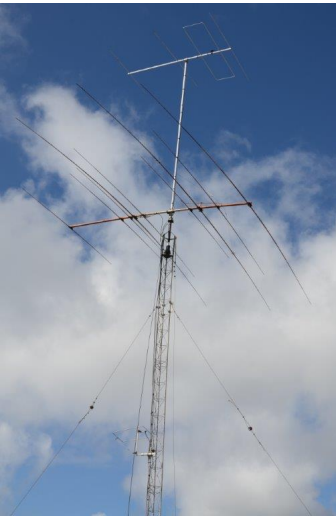
The 4 element 50Mhz LFA-LN installed at ZD7VC
