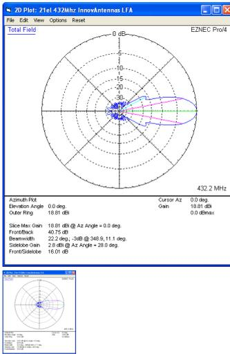
A 21 element super low-noise 432MHz LFA Yagi
