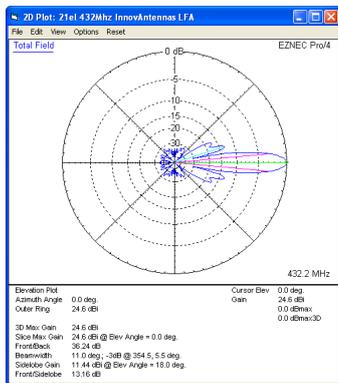
Free space elevation plot of 4 antennas - 1.622V x 1.710H
