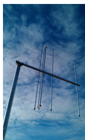
A 4 element low-noise, Marine Band (155MHz - 157MHz) OWL Yagi -
