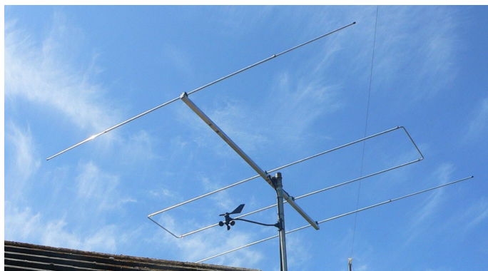
A low-noise 50MHz LFA Yagi
