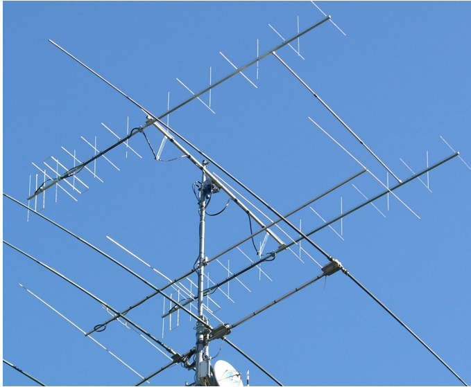
20el LFA Ultra - 144-145MHz for super low noise X-pol Yagi for weak signal operation
