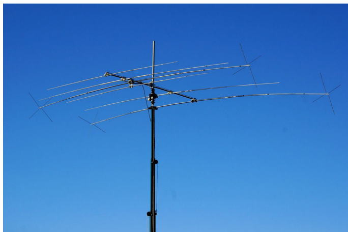
XR3 - 6 element 3 band HF Yagi (20/15/10) with 3.1m boom
