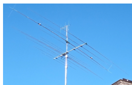
An XR6 below a Delta C-140 Rotating 40m dipole @ OE7MPI
