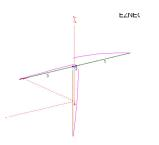
The above shows a Yagi fed with coax and no balun at the point at which the coax is connected. The current distribution is uneven through the driven element and the coax cable can be seen to be radiating too
