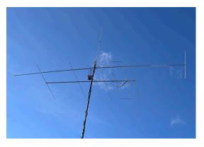
A highly efficient yet very HD 20m/14MHz rotating dipole
