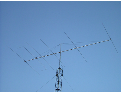
How the OP-DES looks; A 6el 28MHz OP-DES with single taper boom
