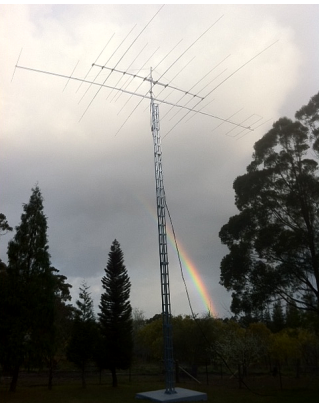
The 8el 50MHz InnovAntennas LFA at VK2IZI
