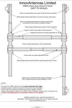
An H frame for 4 x 7el 50MHz LFA-HD Yagis
