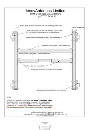
An H frame for 4 x 7el 144MHz LFA Yagis
