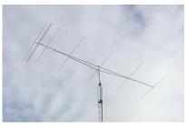
A 7 element OWL Super-Light 50MHz / 6m DX Yagi / low noise Yagi
