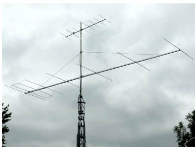
The 7el WOS installed are G2SJX
