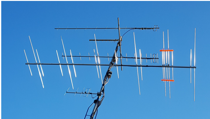
A Dual band 70/144MHz Yagi with single feed point 18 element in total and 4.5m boom
