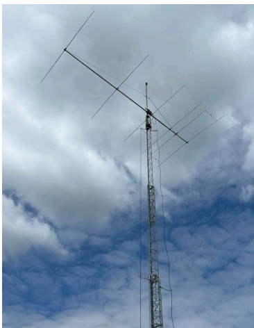
The 6el (set for 28-30MHz) 8.5m OP-DES @ G0FWX installed spring 2022
