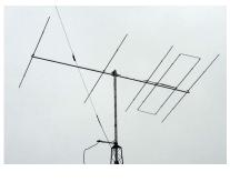
5el 85.5MHz LFA Yagi - Covers 85-86MHz
