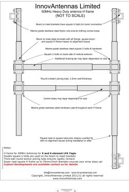
An H frame for 4 x 5el 50MHz LFA Yagis
