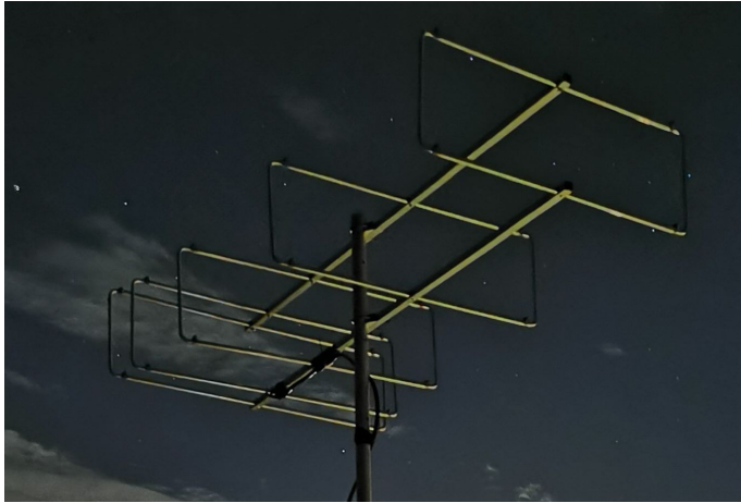
A 5 element High Gain, Super-small 144MHz LFA-Q Quad style Yagi
