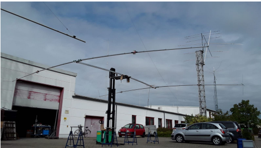
The Delta C-240 without any boom guys to show size and strength.
