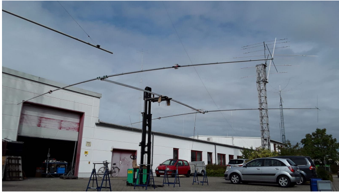
Delta C-240 Compact, HD 40m Yagi. 7m long, 11.5m wide
