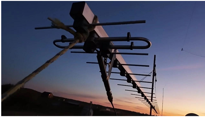
the Best Yagi Antenna for 70cms - A 30 element super low-noise 432MHz LFA Yagi
