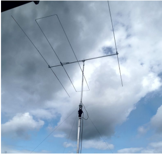
The 3el 28MHz LFA @ G1OVK
