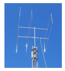
A Super High Gain Quad-style beam antenna for 28Mhz for high power 20KW+
