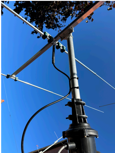
Up close to the feed point with a current balun (InnovAntennas Ferrite Core Balun) installed
