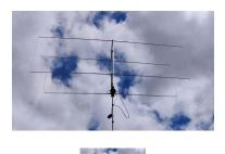
A Super High Gain Quad-style Rigid quad beam antenna for 21Mhz
