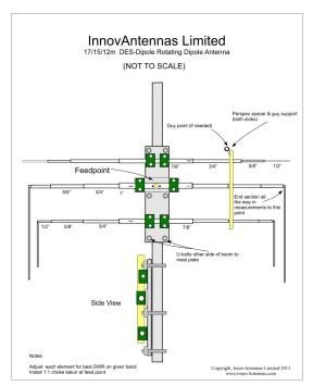
The DES-dipole Antenna Layout
