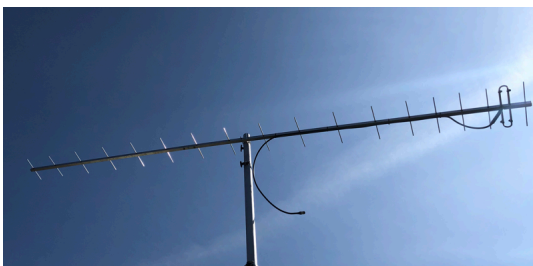
The 18el LFA-Ultra ready for connection to a masthead preamp
