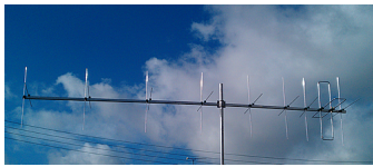
A single 18el (9+9) X-pol LFA Yagi
